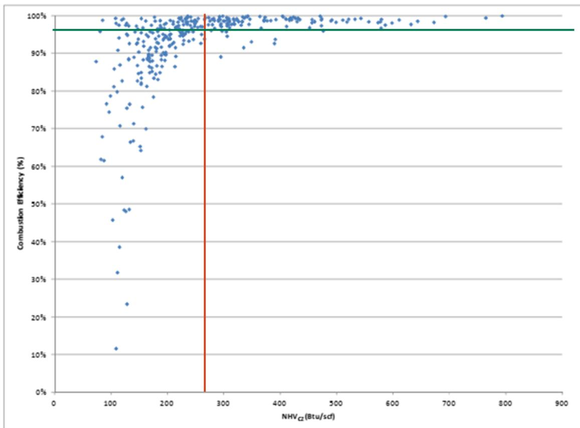
**Figure 1:** Relationship between flare CE and NHVcz as well as regulatory target for CE (>96.5%) and compliance threshold for NHVcz (>270 BTU/scf). Source: Ref. USEPA, 2012, p. 3-33. The red vertical line ( $\text{NHV}_{\text{CZ}}=270 \text{ BTU/scf}$ ) and green horizontal line ( $\text{CE}=96.5\%$ ) are added by author.
