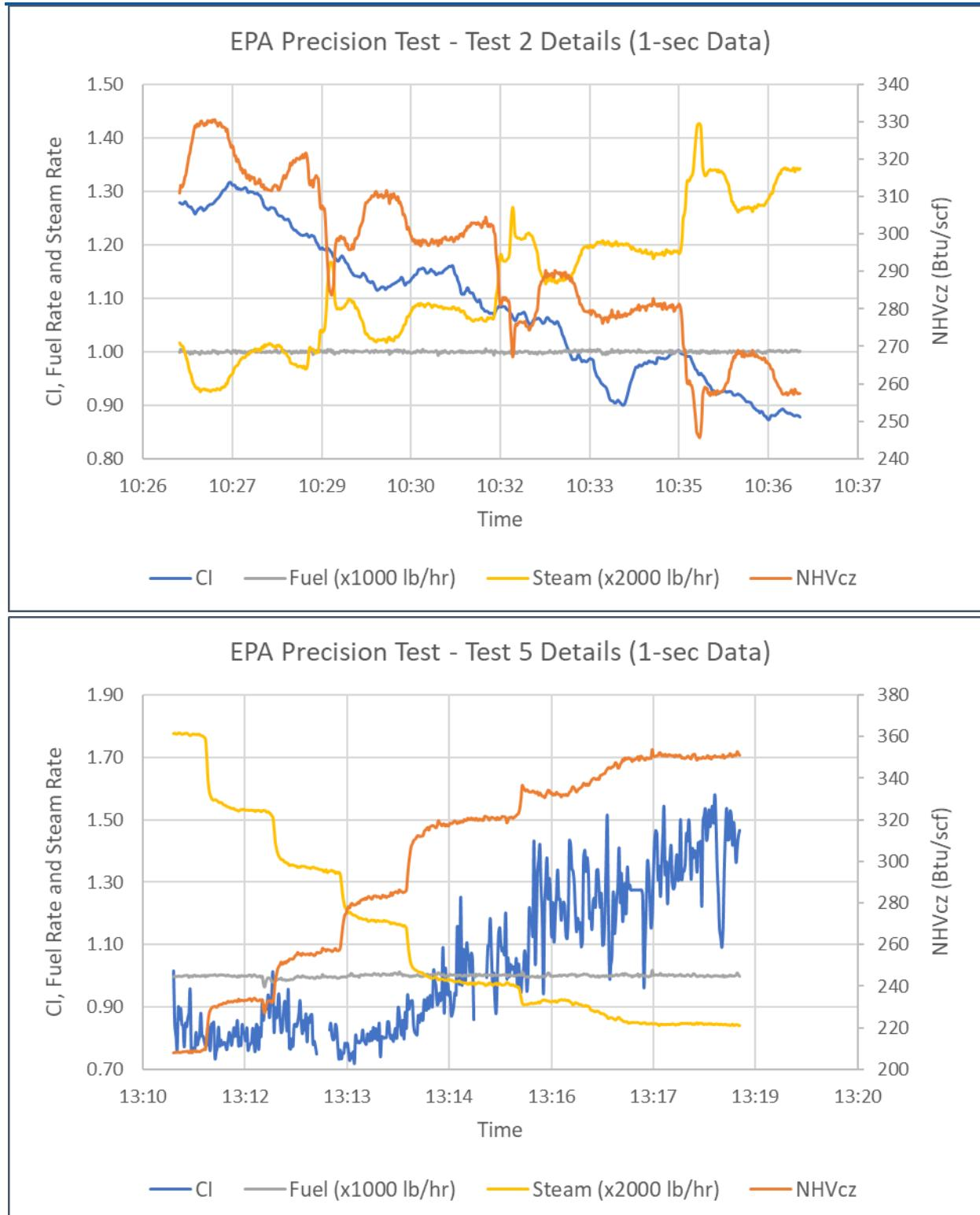
**Figure 5:** Time series plot at 1-second interval for CI, fuel rate, steam rate, and  $\text{NHV}_{cz}$  for EPA Precision Test 2 (transition from high CE to low CE and Test 5 (transition from low CE to high CE).
