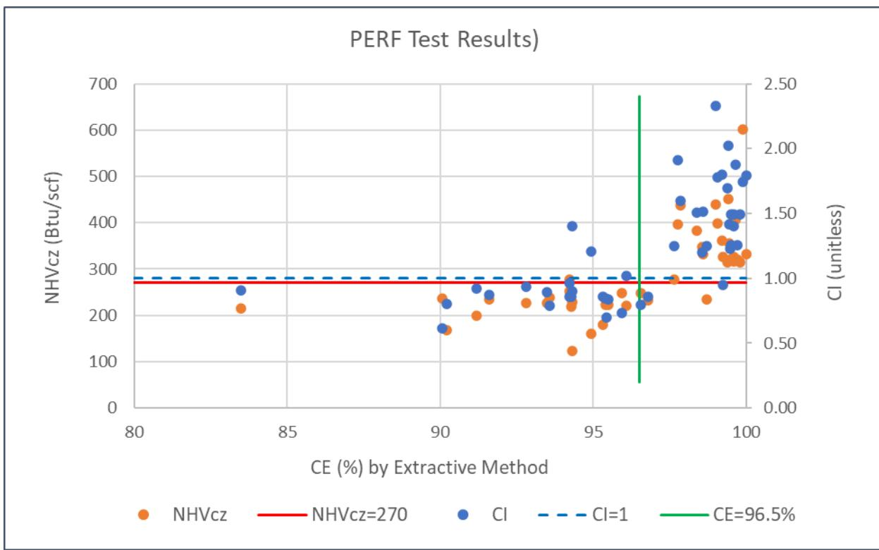
**Figure 6:** Comparison of the NHVcz method and the CI method based on the PERF flare study.
