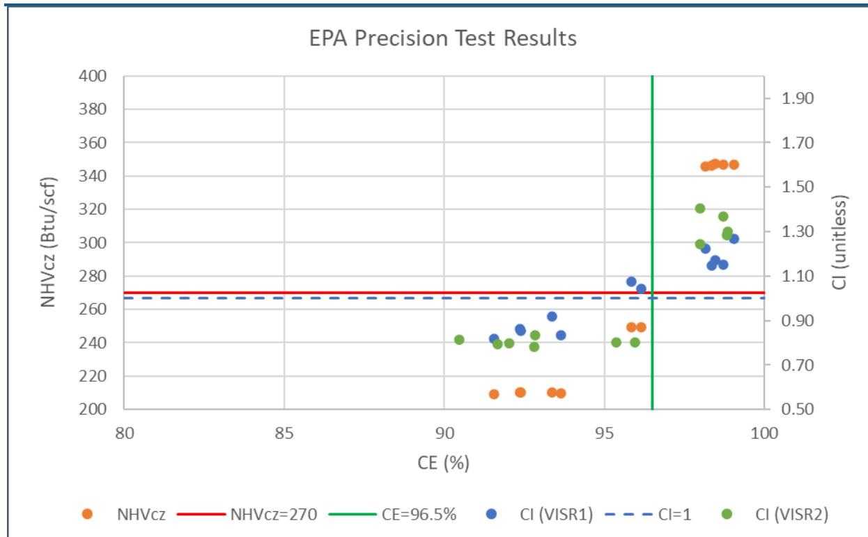
**Figure 2:** Using NHVcz and CI for compliance monitoring – Results based on EPA precision test in 2018.
